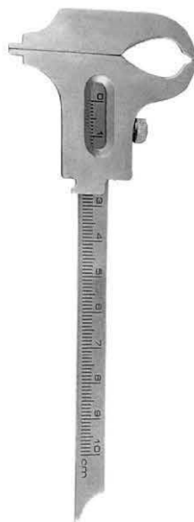
Fig.2 TM-127-1873 Boley Measuring range 0-100 mm
